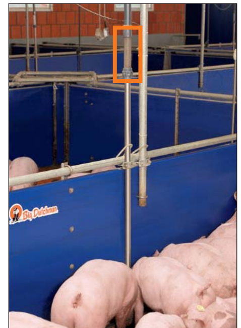
Transparent pipe for feed-flow monitoring
